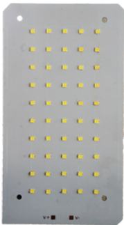
Street Light PCB
